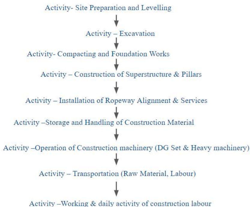
Figure 14. Activities involved in Construction Phase
