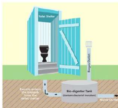
SCHEMATIC DIAGRAM OF BIO-TOILETS
